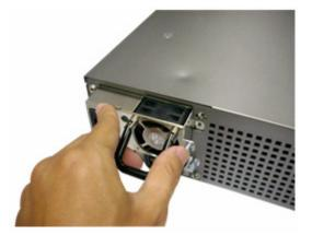
5. Fasten the screw on the power supply in clockwise direction.
