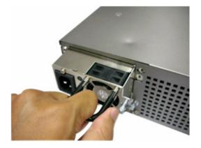
4. Plug in the new power supply to the NAS.
